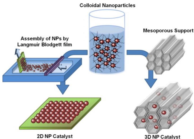
Figure 2. Schematic illustrations for preparation of colloidal nanoparticle-based 2D and 3D catalysts.
