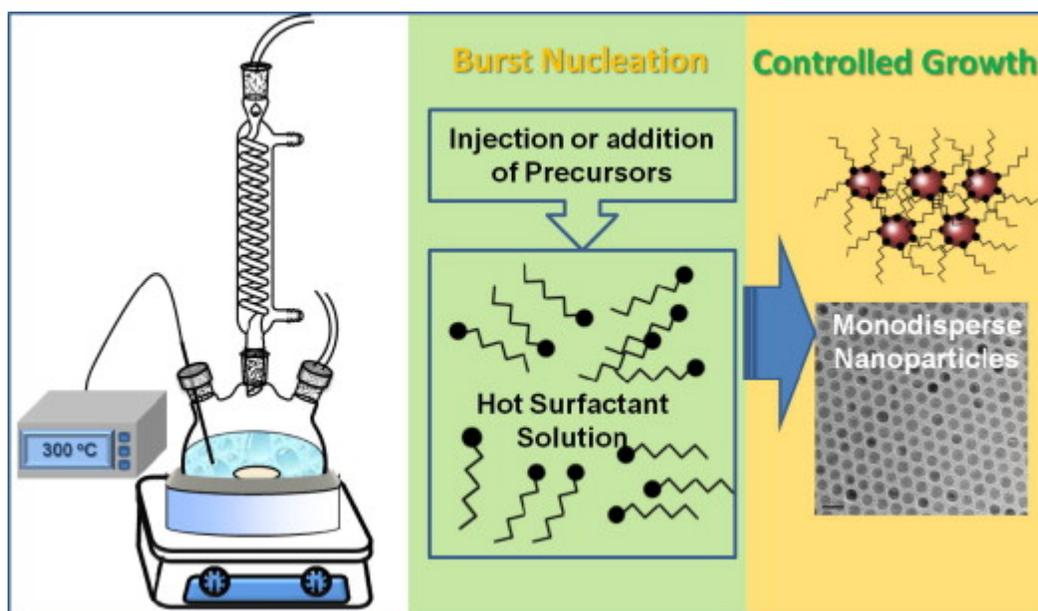
Figure 1. A typical reaction setup and concept for colloidal synthesis of nanoparticles.
